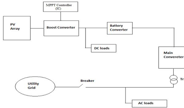
Figure 2: A Compact Representation of Proposed Micro Grid
