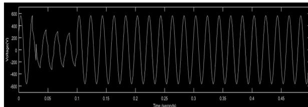
Figure 9: AC Side Voltage of the Main Converter with Variable Solar Irradiation Level and Constant DC Load
