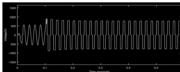
**Figure 12: AC Side Voltage of the Main Converter with Constant Solar Irradiation Level and Variable DC Load**
