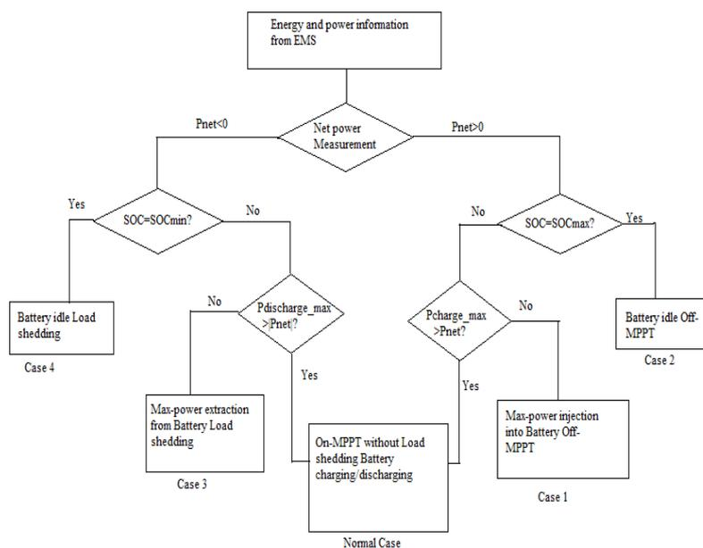
**Figure 3: Control Mode Diagram for the Isolated Micro Grid [28]**
