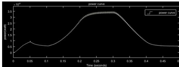
Figure 7: PV Output Power
