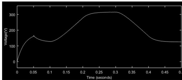
Figure 8: Output Voltage of Boost Converter
