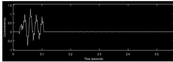
Figure 13: AC Side Current of Main Converter in Isolated Mode
