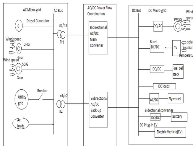
**Figure 1: The AC/DC Micro Grid System**
